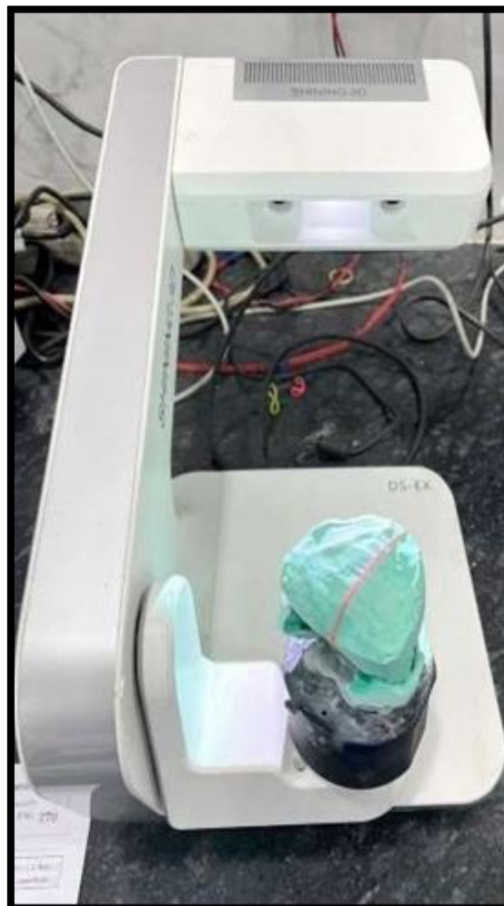
Figure 1: Showing scanning of stone model by shinning 3D scanner to obtain STL files.
