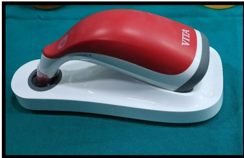
Figure 5: Spectrophotometer (VITA easy shade)
