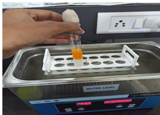
FIGURE 1: Aqueous (AqEO) (bottom) and non aqueous (micelles) (MiEO) (top) in a sonicator water bath (IGene Labserve Pvt. Ltd. New Delhi).
