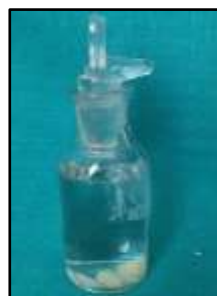
Fig 13 samples were stored in distilled water for 24 hrs. to allow water absorption.
