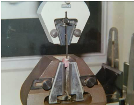
Figure 8:- Testing of specimen in universal instron testing machine
