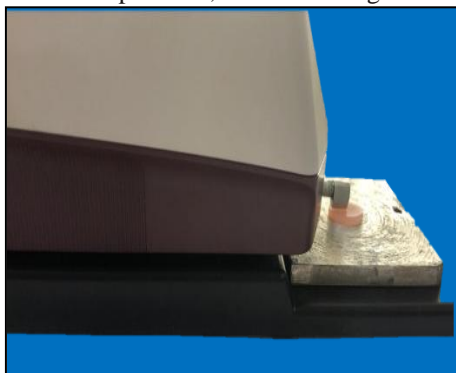
Fig no 3 Measuring surface roughness with surface roughness tester (Mitutoyo)
