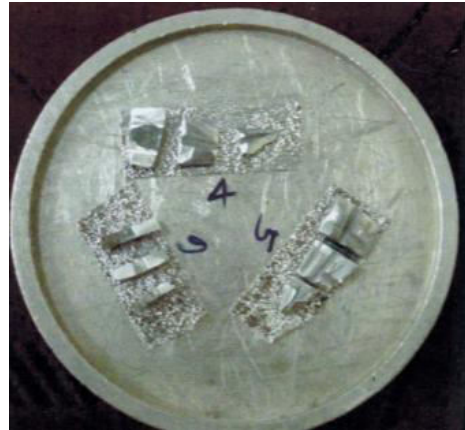
Figure 5: Gold sputter coated sample
