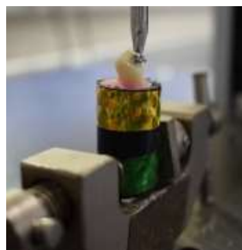
Fig:9- Acrylic jigs placed in Instron Universal testing Machine to test shear bond strength.
