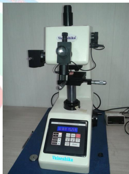
Figure 1: Vickers indenter to measure microhardness
