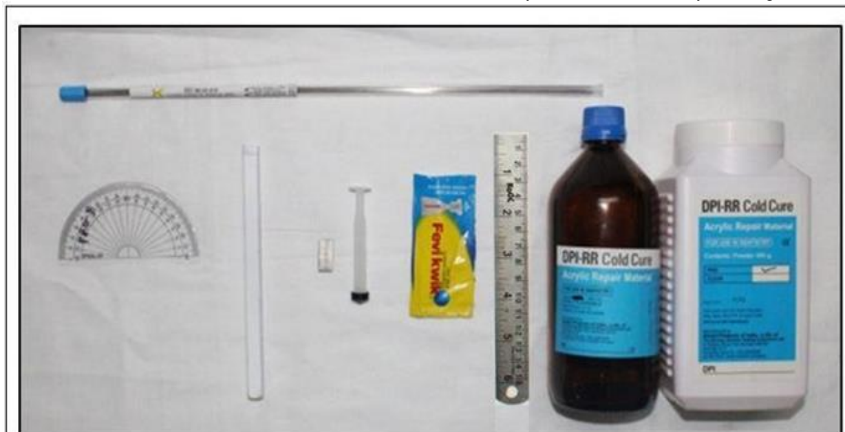
Fig. 2: A simple geometric protractor, an iron metal rod ((15cm l), 0.019 x 0.025 stainless steel straight wire, neodymium iron boron (NdFeB) magnet 2 cm l and 2mm thick, Plunger flange of a disposable plastic syringe, cyanoacrylate adhesive (fevikwik), Short Metal scale (15cm l), DPI-RR Cold cure acrylic (Monomer and Polymer)
