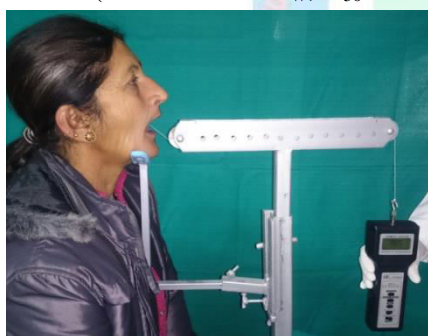
Figure 6: Testing procedure – retention of maxillary denture base being measured on the patient
