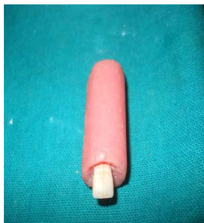
Figure 1: Sample mounted in PVC pipes filled with autopolymerising resins.
