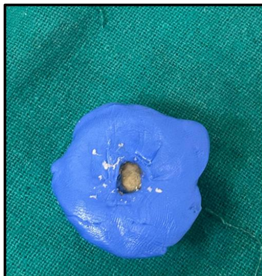
Fig.7-Biodentine added in minor increments in the mold space
