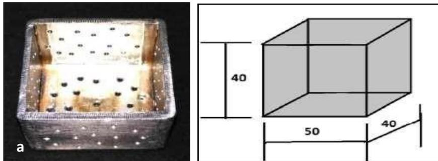
**Custom-made stainless steel perforated metal receptacle**
