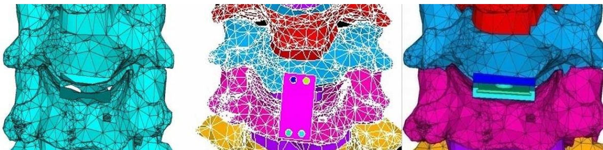
Figure 6: (a) Finite element model of surgically removed bone (b) Finite element model of plate and screw implant (c) Finite element model of artificial disc implant
