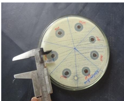
Figure 3: Measurement of zone of inhibition by vernier callipers
