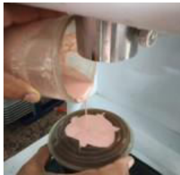
Figure no.(6) Refractory cast poured with ethyl silica bonded investment material.
