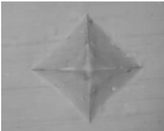
Figure 3 VH indentation on the top surface of SDR
