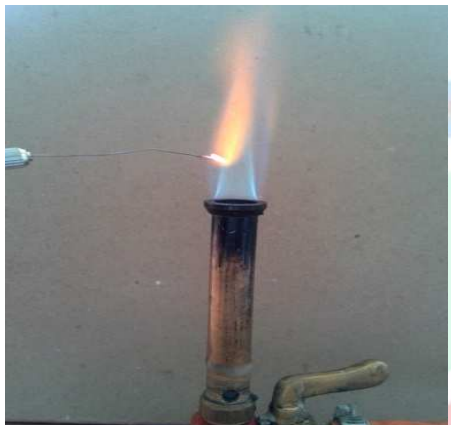
Figure 4: Yellow- red color flame seen on burning of the specimen indicating presence of calcium ions
