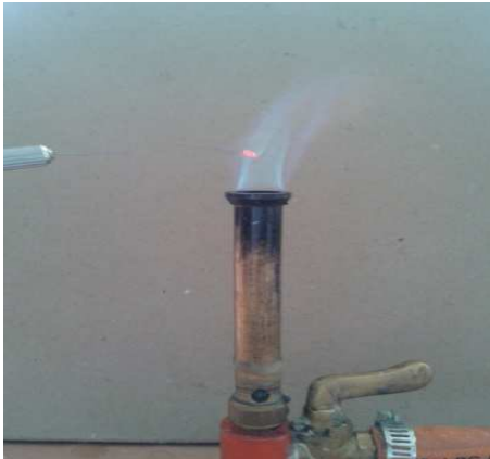
Figure 3: Loop carrying the specimen into the blue part / clear zone of the bunsen burner.
